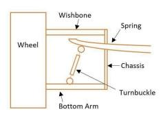
be used to connect the front transverse leaf spring to the upper or lower suspension arm and is solely for the purpose of adjustment to spring rate and ride height, thus, allowing a maximum of three rose joints to each front suspension unit but only if the turnbuckle is used in this way.
