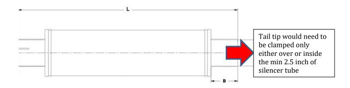
L = max 29 inches, min 18 inches B = max 8 inches, min 2.5 inches, both ends
