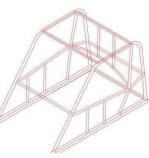
bar/door bars to the chassis and be constructed with a minimum of 25mm tube or 25mm x 25mm box section and be equally spaced between the front and side/intermediate hoops. (See drawing for minimum structural requirements).
